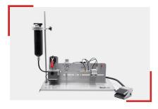
The Tridak® Model 1001 fills syringes, one at a time, quickly and accurately from a material reservoir. It is ideal for low-volume production or as an alternative to filling syringes manually.
