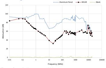
Test performed with a two-coat thickness.
